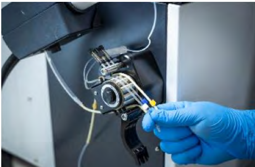
Figure 15. Pump tubing must be compatible with the solvent you are using.
