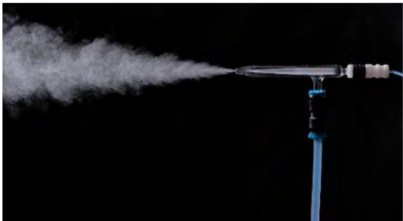
Figure 12. Samples are typically introduced in liquid form for measurement using any atomic spectroscopy technique. All techniques, except GFAAS, use a nebulizer to turn the liquid sample into an aerosol mist. GFAAS injects the liquid sample using a syringe.
