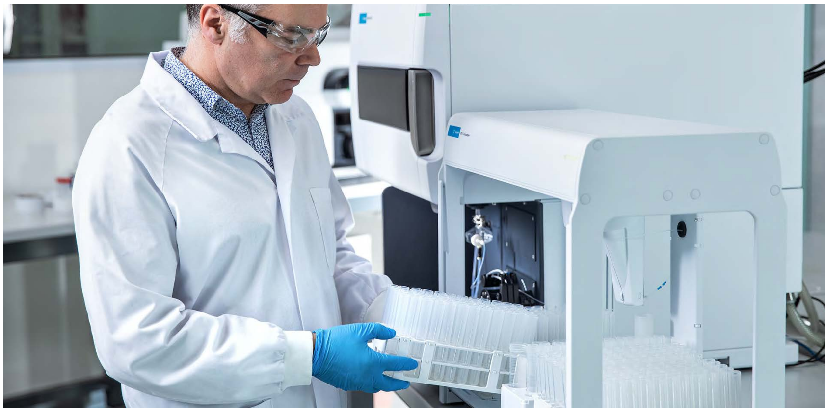
Figure 9. Using an autosampler will increase productivity and allow the instrument to run unattended.
